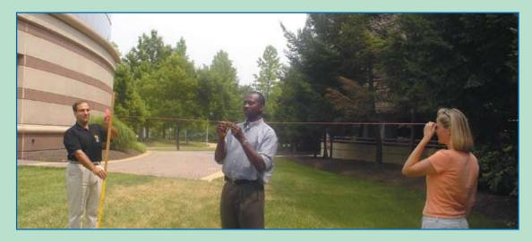
After you have completed at least 4 transects or lines from the center (position of person #2), plot each transect on a sheet of graph paper with the length being the x axis and the elevation being the y axis. Refer to Figure 5. The line on the graph demonstrates to you the high and low spots across the bottom of the garden site. This will help determine the soil removal or additions to get a level ponding area.
